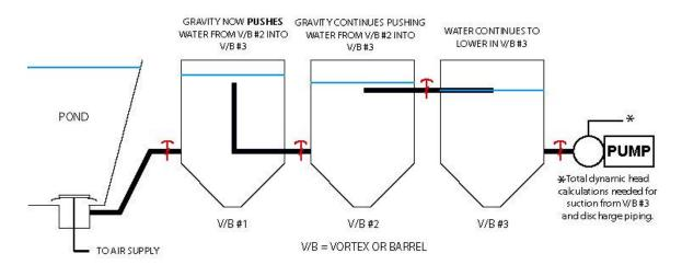
THE CHAIN REACTION CONTINUES, WITH THE WATER LEVEL LOWER IN V/B #2 WATER FROM V/B #1 IS NOW PUSHED INTO V/B #2. THE LARGEST FORCE STOPPING ALL THIS FROM HAPPENING INSTANTLY IS FRICTION, WHAT WE LEARNED EARLIER ABOUT FRICTION IN PIPING CAN NOW BE APPLIED TO THE GRAVITY FLOWING WATER THROUGH THE V/Bs.
