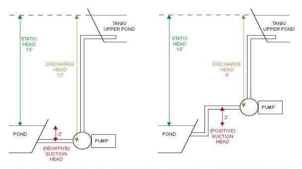
Note: Suction head and discharge head should = static head. Take note in the case of the flooded suction pump suction head would be a negative number.
