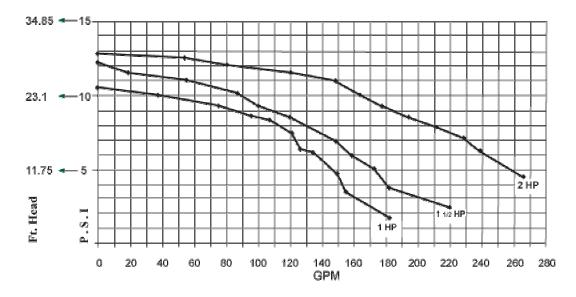
The pumps come with 2 1/2" unions for IN and OUT. A 2 1/2" pipe will give you higher pressure, but the flow will slightly decrease. You must increase to 3" pipe to get 100% max flow. This will not overamp the motor; and will match the performance curve we have provided.
