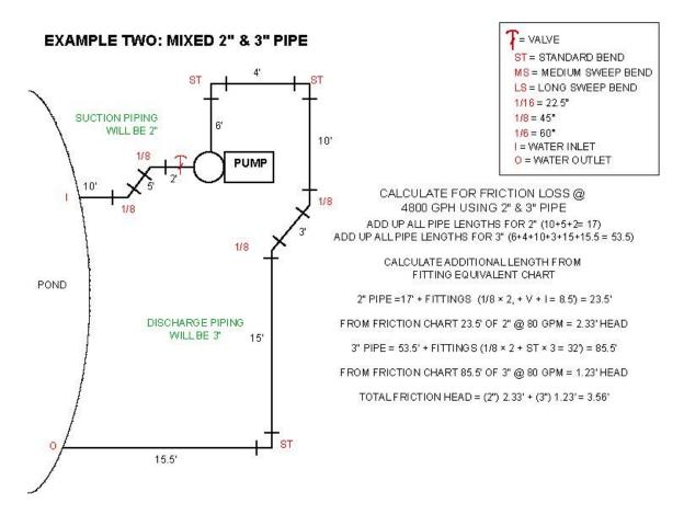
In the above example 2" was used for the suction end, and 3" for the discharge. The head was calculated for the 2" section, and then for the 3" section and then both added together.
