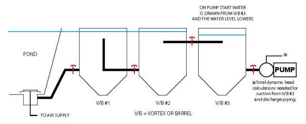
AS THE WATER LEVEL LOWERS IN V/B #3 AN IMBALANCE IS CREATED LEAVING THE WATER IN THE FIRST TWO V/Bs & POND HIGHER.
