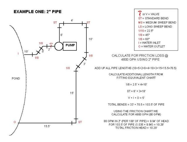
Hopefully the above drawing explains how to add lengths of pipe and calculate in fittings. It may help to have the friction loss chart printed out and available while viewing these.
