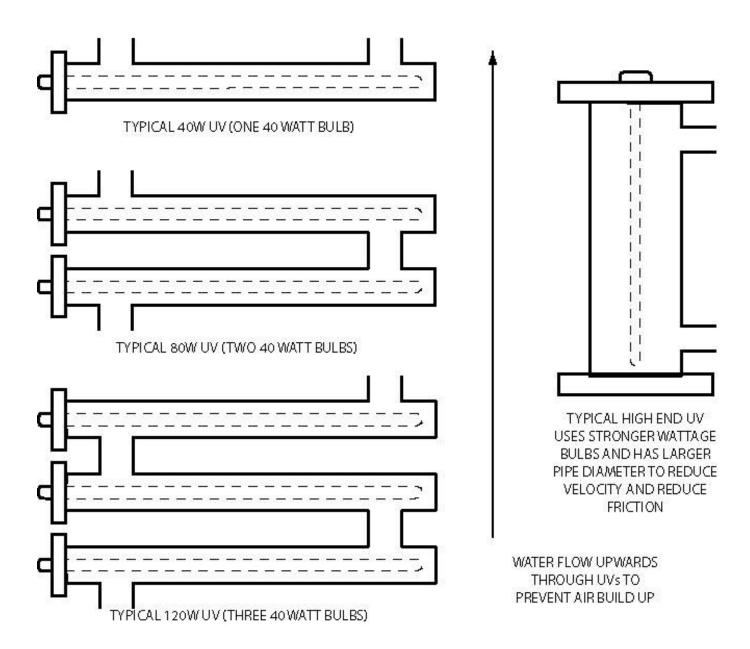
Looking at the cheaper units and all the 90° bends, you can see why they are very restrictive to flow. Couple that with the lost inner space, and they are an extreme bottleneck. I've always installed UVs with unions, and made a piece of pipe with unions to take its place. That way for the times of year when they're not necessary, they can be taken out of the system.
