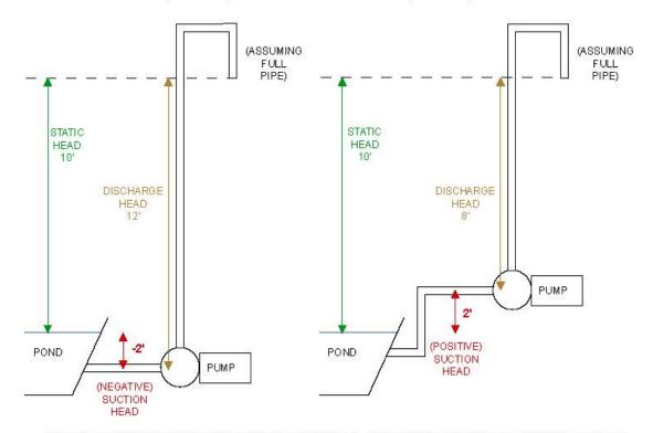
Note: Suction head and discharge head should = static head. Take note in the case of the flooded suction pump suction head would be a negative number.
