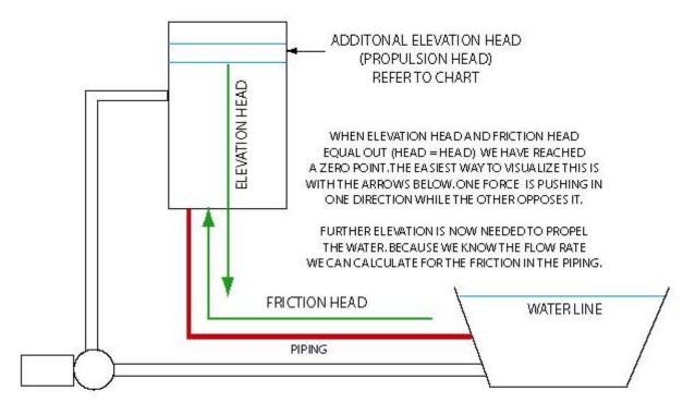
A KEY POINT TO REMEMBER IS THAT WHEN THE PUMP STARTS IT WILL LOWER THE WATER LEVEL IN THE POND TO FILL THE TANK. VICE VERSA WHEN THE PUMP SHUTS OFF IN THIS SCENARIO THE TANK WILL CONTINUE TO DRAIN BACK INTO THE POND POSSIBLY OVERFLOWING IT.
