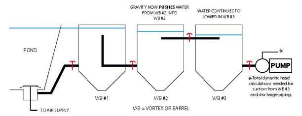
AS THE WATER CONTINUES TO LOWER IN V/B #3 THE FIRST GRAVITY MOVEMENT STARTS. WITH THE DOWNWARD FORCE OF GRAVITY PUSHING ON THE ALL WATER THE WATER IN V/B #2 STARTS TO MOVE. THERE HAS TO BE A WATER LEVEL DIFFERENCE FOR THIS TO HAPPEN, SO EVEN THOUGH V/B #2 IS SUPPLYING V/B #3 IT MUST BE LOWER IN LEVEL TO MAINTAIN THIS FLOW.
