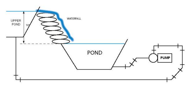
In this example we pump to an upper pand which will flow to the lower pand. With all piping below ground we concentrate again on static elevation head. Remember from our earlier examples this is measured from water line to water line. The 10' can be added again to any of the piping calculations to give Total Dynamic Head.
