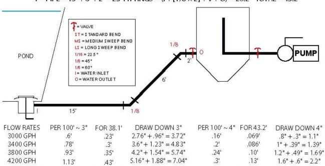
The first number in draw down is friction from the piping and the second is the elevation needed for propulsion.
